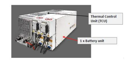
\* Primove" is Bombardier's vehicle battery system
