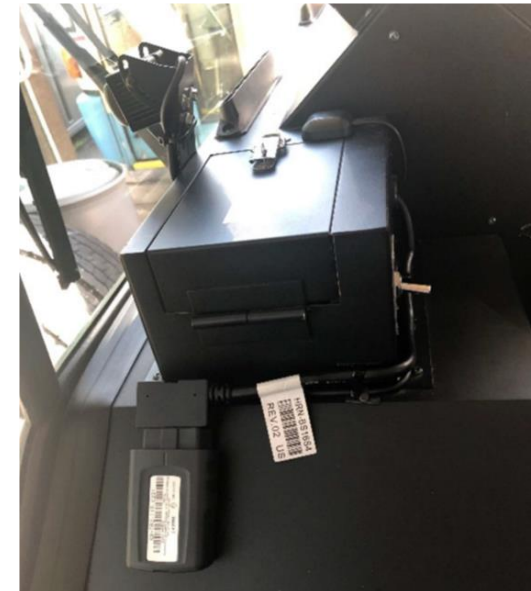
GPS logger installed at bus front
